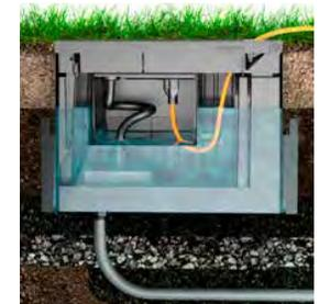
Outdoor Ground Box, exterior view, view installed with bricks, and a cross-sectional view of a Ground Box installation.
