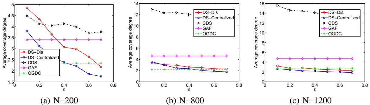
Fig. 8. Average coverage degree as a function of  $\epsilon_0$ . Sensors are uniformly distributed in a  $40m \times 40m$  square region.  $t_{max} = 8$  and  $s = 4$ .
