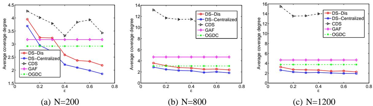
Fig. 11. Average coverage degree as a function of  $\epsilon$ . Sensors are non-uniformly distributed in a  $40m \times 40m$  square region.  $t_{max} = 8m$  and  $s = 4m$ .
