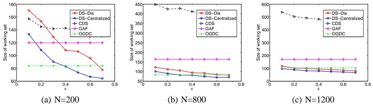
Fig. 7. Size of working set as a function of  $\epsilon_0$ . Sensors are uniformly distributed in a  $40m \times 40m$  square region.  $t_{max} = 8$  and  $s = 4$ .
