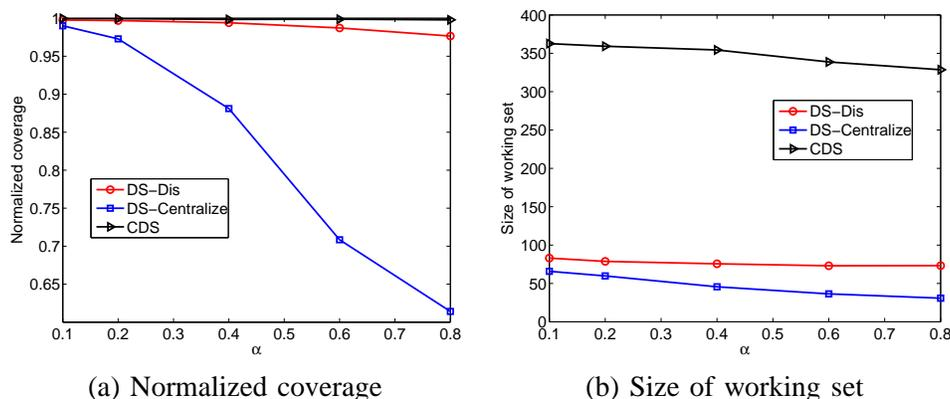
Fig. 13. Isotropic sensors: coverage and size of DS as functions of  $\alpha$  with  $N = 800$  sensors uniformly distributed in a  $40m \times 40m$  square region.  $\epsilon_0 = 0.6$ ,  $t_{max} = 8m$  and  $\bar{s} = 4m$ .
