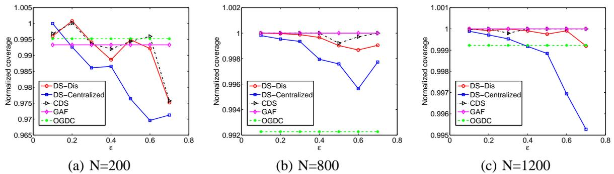
Fig. 6. Coverage as a function of  $\epsilon_0$ . Sensors are uniformly distributed in a  $40m \times 40m$  square region.  $t_{max} = 8m$  and  $s = 4m$ .
