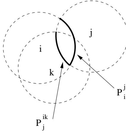
Fig. 2. Union of disks.  $P_i^j$  and  $P_j^{ik}$  are the lengths of the circle arc in the boundaries of  $B_i$  of  $B_j$ 's side of the bisection and the arc on  $B_j$  segmented by the bounding circle of  $B_i$  and  $B_k$ .
