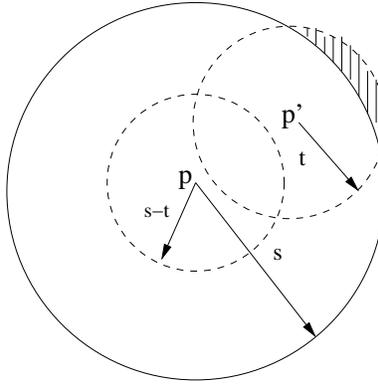
Fig. 3. Considerations to tighten the sufficient condition. If there is no node in the shaded area,  $p$  is covered.
