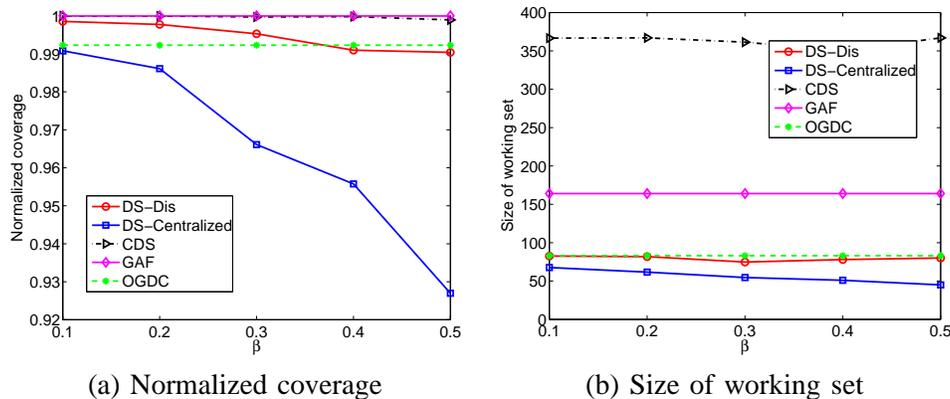
Fig. 12. Coverage and size of DS as functions of variation in transmission power control parameter  $\beta$  with  $N = 800$  sensors are uniformly distributed in a  $40m \times 40m$  square region.  $t_{max} = 8m$ ,  $\epsilon_0 = 0.6$  and  $s = 4m$ .
