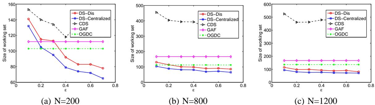
Fig. 10. Size of working set as a function of  $\epsilon$ . Sensors are non-uniformly distributed in a  $40m \times 40m$  square region.  $t_{max} = 8m$  and  $s = 4m$ .
