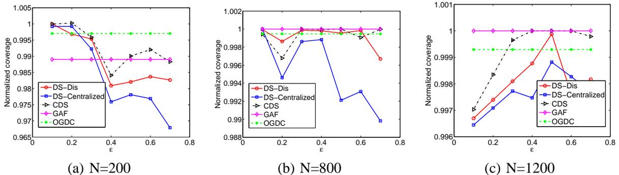
Fig. 9. Coverage as a function of  $\epsilon$ . Sensors are non-uniformly distributed in a  $40m \times 40m$  square region.  $t_{max} = 8m$  and  $s = 4m$ .
