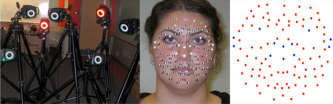
Fig. 2. The left shows a facial motion capture system, the middle is a snapshot of the captured actress. In the right panel, blue and red points represent the 102 captured markers, where the red points are the 90 markers used for this work.
