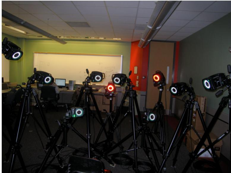
Figure 1. A VICON motion capture system
