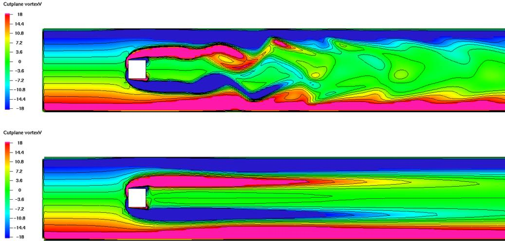
Figure 12: Problem Q2 ( $Re=100$ ): Spanwise vorticity at time  $t=16$  for the midplane  $y = 0.205$ . The top plot shows the development of vortex street for solution by BDF2 with FD advective terms; the bottom plot shows an over-diffusive solution computed by BDF2 with semi-Lagrangian method (linear interpolation). Both solutions were computed with  $h_{\max} = 1/256$  and  $h_{\min} = 1/1024$  at  $t = 16$ .
