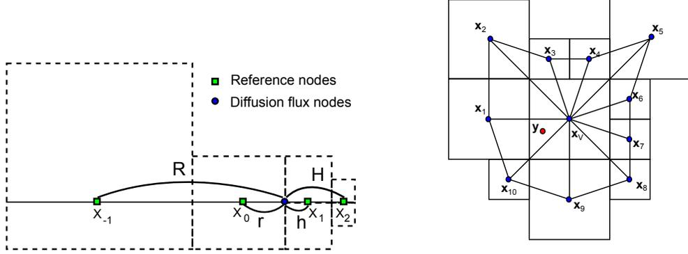
Figure 5: Left: Reference points for the diffusion flux approximation; Right:  $u_h(\mathbf{y})$  is defined by a linear interpolation based on the fan triangulation with the center in  $\mathbf{x}_v$ , i.e. interpolation of  $u_h(\mathbf{x}_v)$ ,  $u_h(\mathbf{x}_1)$ ,  $u_h(\mathbf{x}_{10})$  in this example.
