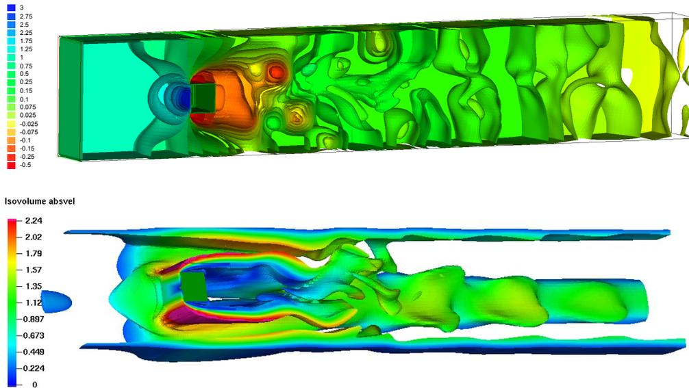
Figure 15: Problem Q2 ( $Re=100$ ): Pressure isosurfaces and vorticity isosurface  $|w| = 20$  colored by the absolute velocity. The plots illustrate solution computed with  $h_{\max} = 1/256$  and  $h_{\min} = 1/1024$  at  $t = 16$ .
