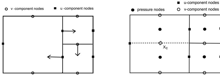
Figure 3: Left: A single local div-free mode, which is subgrid for the coarse grid cell. Right: Introducing additional pressure d.o.f. for the coarse cell next to fine cells. This yields a stronger discrete div-free condition and precludes the occurrence of subgrid div-free modes such as shown in the left figure.
