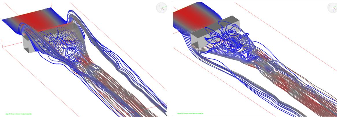
Figure 14: Problem Q2: Streamlines of the developed flow around a square cylinder for  $Re=100$ . The streamlines are selected for two fluid layers entering the domain slightly above and below  $x = 0.21$ .
