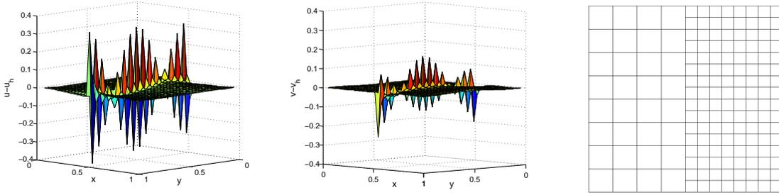
Figure 2: The velocity error is dominated by the div-free modes occurring on the coarse-to-fine grids interface. The left figure shows the  $u$ -component of the error, the middle figure shows the  $v$ -component, and the right figure shows the grid for  $h = 1/8$ .
