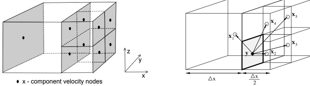
Figure 1: Left: Each shared face holds a node for velocity  $x$ -component. The nodes are located at faces barycenters. Right: Discretization stencil for  $\partial p/\partial x$ .
