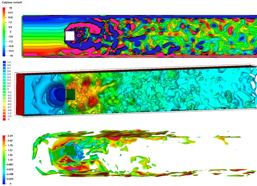
Figure 17: Channel flow around a square cylinder at  $Re=10000$ : Spanwise vorticity for the midplane  $y = 0.205$ . Pressure isosurfaces and vorticity isosurface  $|\mathbf{w}| = 100$  colored by the absolute velocity. The plots illustrate solution computed with  $h_{\max} = 1/256$  and  $h_{\min} = 1/1024$  at  $t = 8$ .
