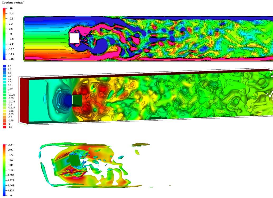
Figure 16: Channel flow around a square cylinder at  $Re=1000$ : Spanwise vorticity for the midplane  $y = 0.205$ . Pressure isosurfaces and vorticity isosurface  $|\mathbf{w}| = 100$  colored by the absolute velocity. The plots illustrate solution computed with  $h_{\max} = 1/256$  and  $h_{\min} = 1/1024$  at  $t = 8$ .
