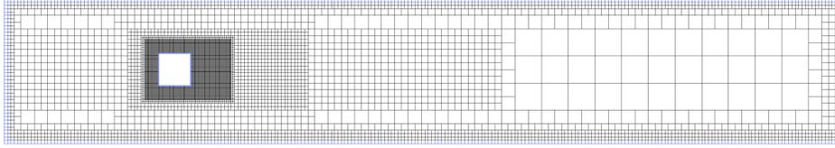
Figure 10: The cutaway of the grid at  $y = 0.205$  for  $h_{max} = 1/32$  and  $h_{min} = 1/1024$ .
