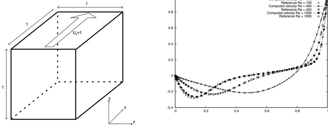
Figure 6: Left: The 3D driven cavity problem setup; Right: The centerline  $((0.5, 0.5, z), 0 \leq z \leq 1)$   $u$ -velocities compared to reference data from [33]
