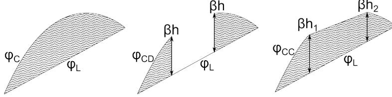
FIG. 3.5. Filled region denotes a correction to the original linear interpolation  $\varphi_L$ . Left picture shows the original cubic interpolant  $\varphi_C$ . Middle picture shows the discontinuous limiting of the cubic correction  $\varphi_{CD}$ . Right picture shows the continuous limiting of the cubic correction  $\varphi_{CC}$ .
