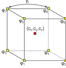
FIG. 3.4. Illustration for the cube with the side of the size  $h$  and the center  $(c_x, c_y, c_z)$  (red box) and variables defined at vertices of the cube  $\varphi_{1\dots 8}$  (yellow boxes).
