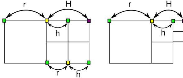
FIG. 3.3. The node marked by yellow box is the current node  $i$  of type A. Green boxes are the nodes that are  $i - 1$  and  $i + 1$  immediate neighbors in the given direction  $Ox$ . Purple boxes mark the  $i + 2$  non-immediate neighbor node.
