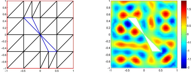
FIG. 6.6. *Example 2: The computational domain  $\Omega$  and the simplicial triangulation  $\mathcal{T}_h(\Omega)$  for the PWDG method (left; the sound-soft scatterer is shown in blue). The substitute solution  $u_s$  computed by the adaptive Interior Penalty Discontinuous Galerkin method from [12] (right).*
