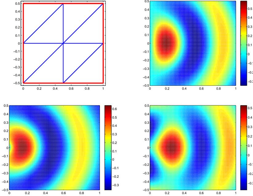
FIG. 6.1. *Example 1: The computational domain  $\Omega$  and the simplicial triangulation  $\mathcal{T}_h(\Omega)$  for the PWDG method (top left). The exact solution for  $\xi = 1$  (top right),  $\xi = 2/3$  (bottom left), and  $\xi = 3/2$  (bottom right).*
