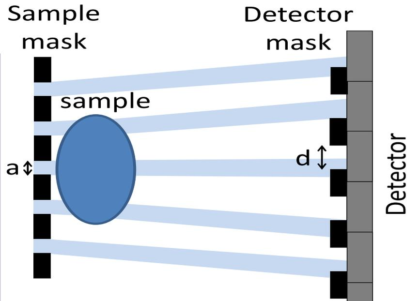
An edge-illumination effect is created using a pair of mutually displaced masks
