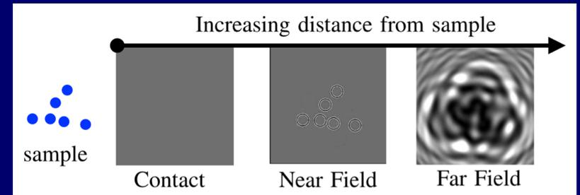
Wave-front distortions due to the object leads to intensity modulations
